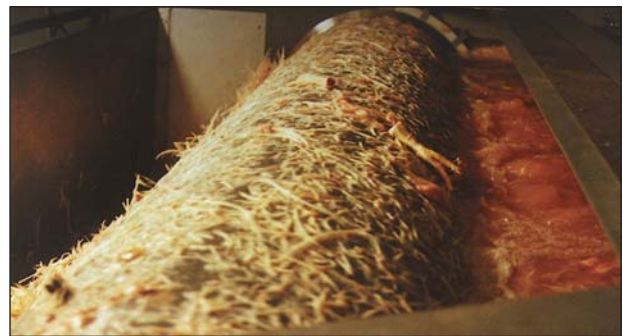
Poultry slaughterhouse - 0,5 mm. Heavily loaded water with large solids: feet, feathers, viscera.
