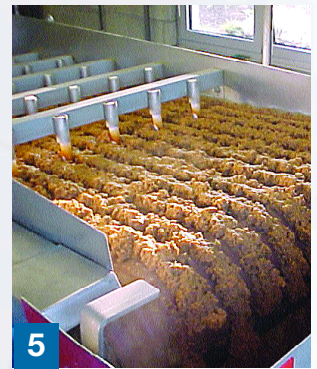
5 Raws of baffles for sludge draining and distribution
