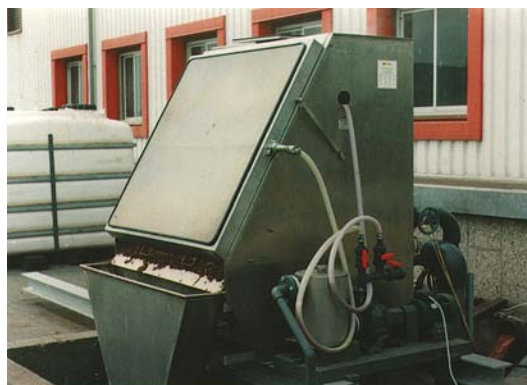
Slaughterhouse raw sewage - Stainless 554 - 48" frame. Rotating front and rear spray system with cover.
