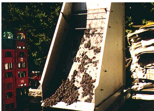
Screening of wine industry rejects. Stainless 254 - 24" frame on bottom belt.
