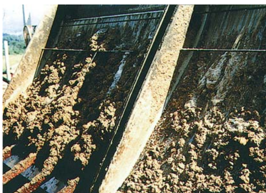
Thickening of paper millstock. 2 x 48" stainless 554 frame.
