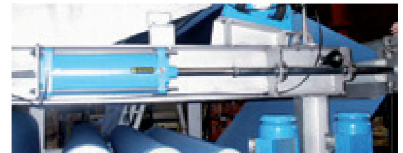
Optional: Wire tensioning via air cylinders
