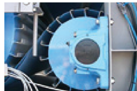
Efficient drainage rolls to minimize rewetting
